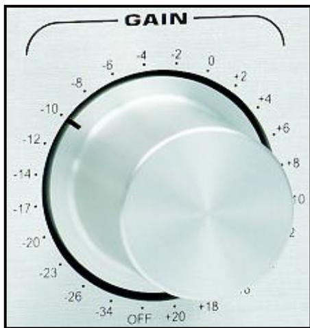
With stepped attenuators, each switch position is for a precisely calculated voltage divider, so front panel calibration markings represent actual signal levels.
